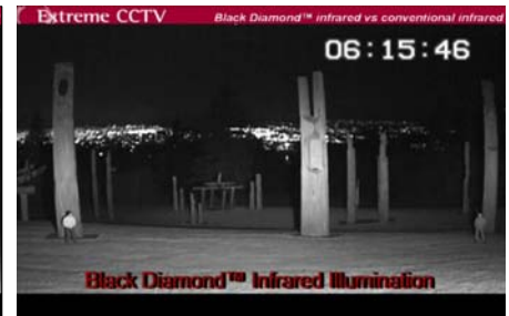
Above: Conventional infrared illumination yields a washed out image (above left) with a high-noise darkness around a bright center. Video analytic software requires high-definition, evenly illuminated scenes such as that shown (above right) through an Extreme CCTV EX85 with Black Diamond™ technology.
