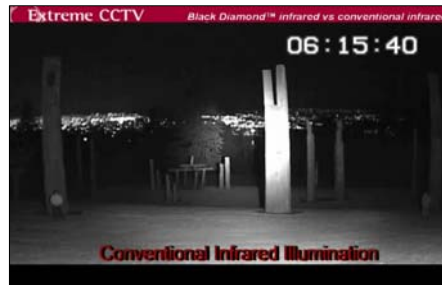
Above: Conventional infrared illumination yields a washed out image (above left) with a high-noise darkness around a bright center. Video analytic software requires high-definition, evenly illuminated scenes such as that shown (above right) through an Extreme CCTV EX85 with Black Diamond™ technology.
